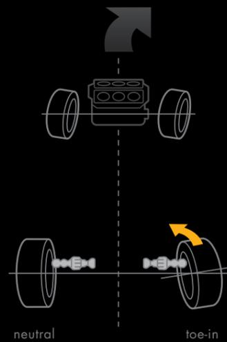
While cornering, both rear wheels are out of phase, making handling agile, precise, and smooth.
