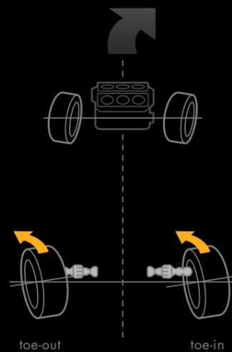
During high-speed lane changes, rear wheels are in phase for enhanced response and stability.
